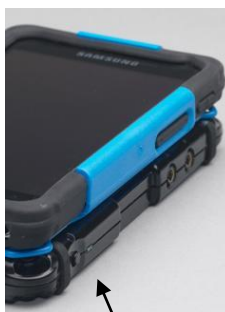
Amp Power Switch
